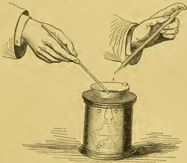
Arrangement for estimating the amount of sugar by the cupro-potassic solution.
